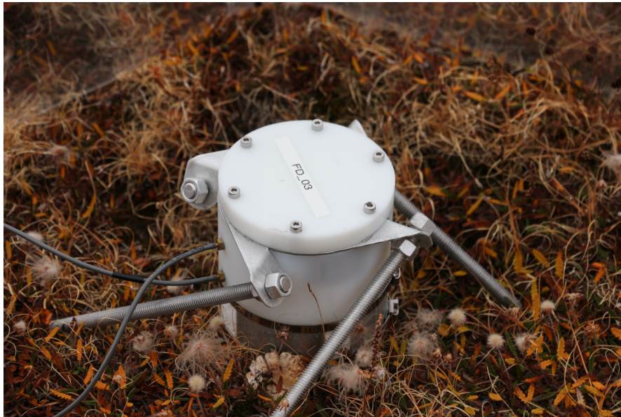
Figure 3.6: One of the FD chambers during field use in Endalen. The two cables on the left-hand side are leading to the power supply and data logger. Below the cables, one of the four membranes is visible.
