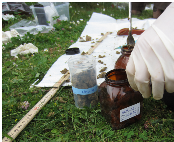
FIG. 2.3 All samples were loosely homogenized with a stainless steel spoon. An aliquot of each soil sample was packed on site for the laboratory on Braunschweig, another one for the laboratory in Vienna.
