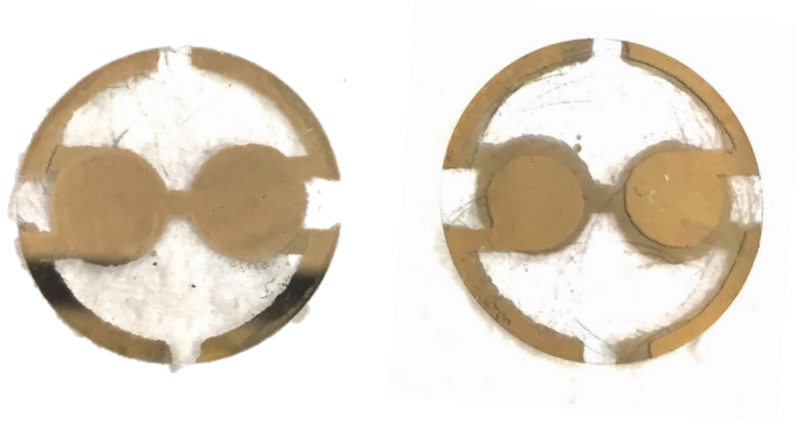
Figure 2.3: QCM wafer with two-electrode system for use in microsensing
