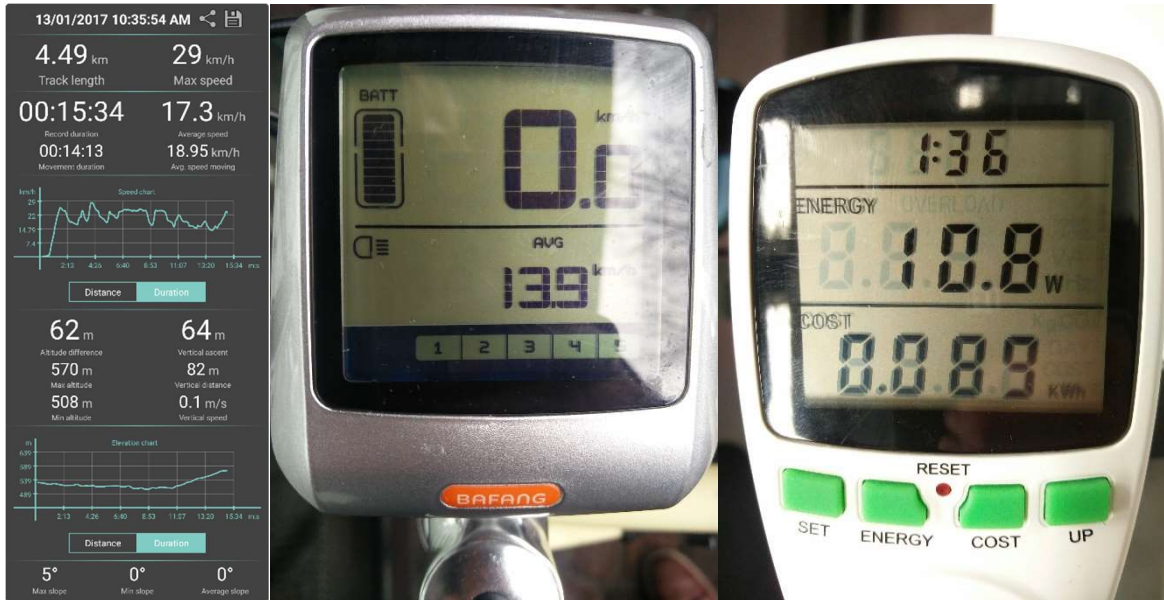
Figure 38: A screenshot from “Geo Tracker”, one of the smartphone applications available ( first picture ). It displays the average velocity of the trip. The second picture shows the average velocity measured by the internal torque sensor on the display of the e-bike itself. The third picture shows separate energy cost meter. The display plots i.a. the measured amount of energy during recharge [kWh]. Since I started each Test Drive with a fully charged battery, the measured value in recharge mode at the respective target location corresponds to the energy consumption of the driven route.
