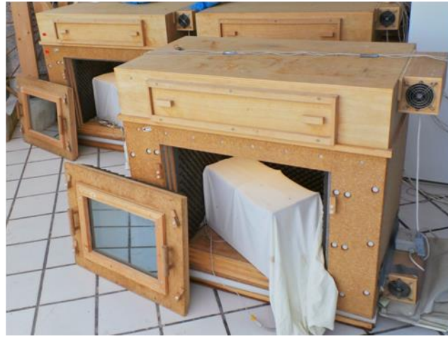
Figure 4. Cage in the Soundproof-Box to be isolated from the outside environment.
