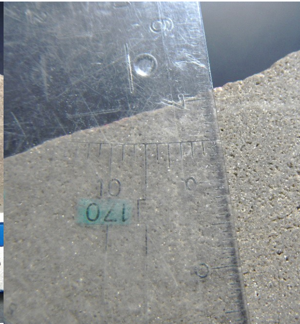
Figure 92: A closer look reveals large pores between the crystalline grains even to the unaided eye.
