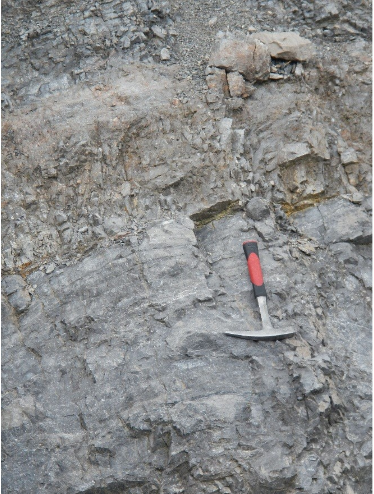
Figure 17: A closer look: Strain partitioning on Keuper bed (thin brown layer between reddish and grey beds) and bedding-controlled fracture density with FDC2 in the lower laminated bed (hammer) and FDC4 in the overlying reddish bed.
