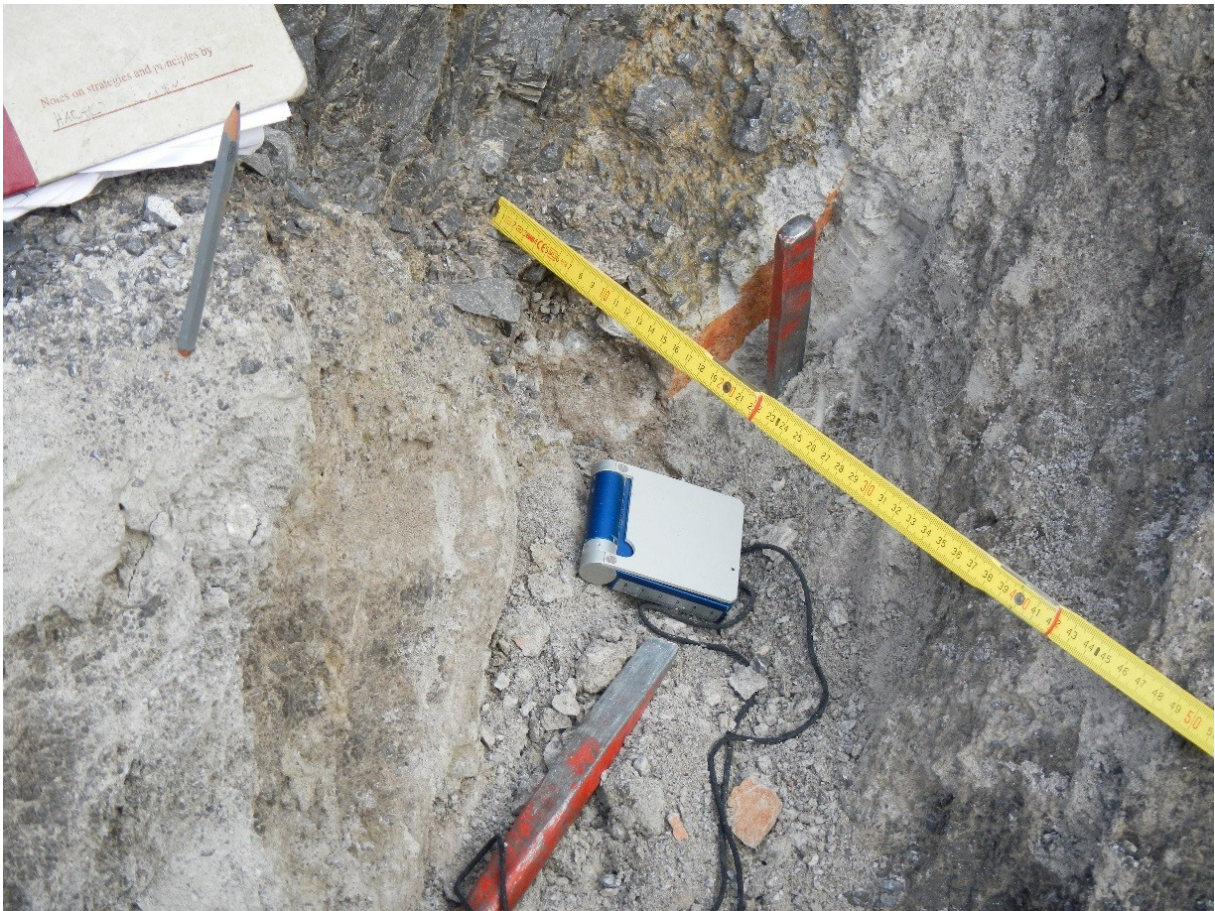
Figure 77: While soft enough at the surface to stick in a pencil, the cemented rock had to be chiseled to remove a sample after digging through around 40 cm of the “kakirite” to the “cataclasite” hidden beneath.
