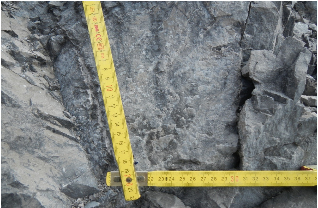
Figure 26: Synkinematic fiber crystals on the footwall of a fault oriented 333/62 with a slickenside 302/59 indicating reverse faulting (view direction SE).
