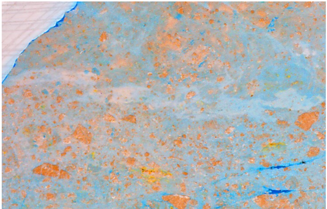
Figure 83: The trace of a former principal slip surface in sample 5.2 (see also in the section of sample 5.2) is not a sharp plane at closer look: The fine grained, white material shows blurred and wavy structures that resemble such produced by liquefaction of loose sediments (length of lower picture edge is 2 cm).
