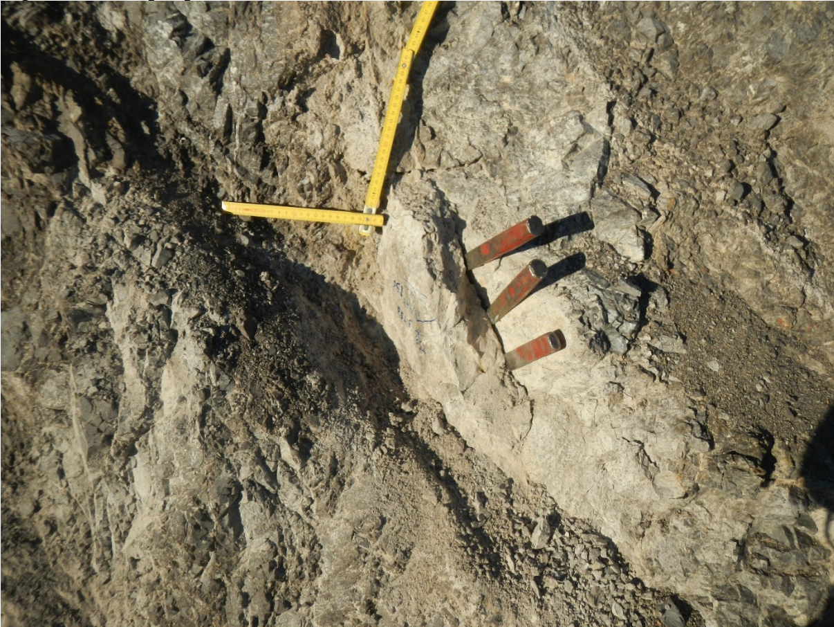
Figure 19: Careful removal of oriented sample using a set of flat wedges (sample 5.2).
