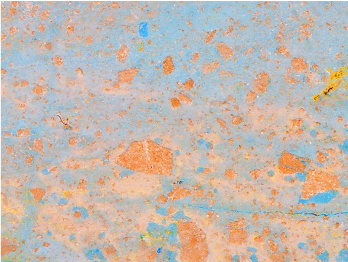
Figure 58: Spotty porosity distribution: Long side = 2 cm, saturation enhanced
