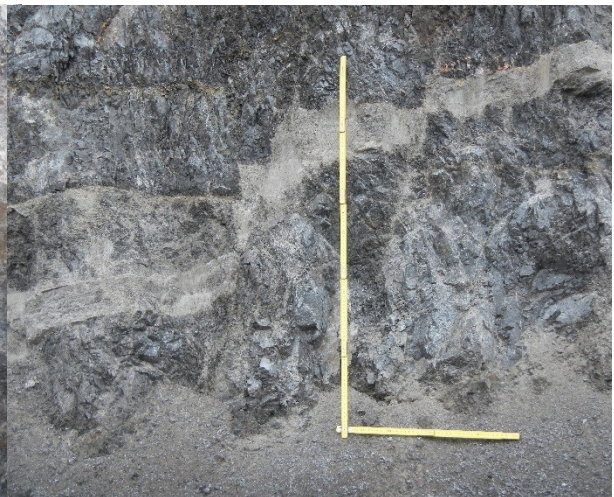
Figure 32: NE dipping normal faults offsetting marker beds and flats of category 1 faults in the south-eastern quarry walls. Height of wall = 30 m, view towards SE.
