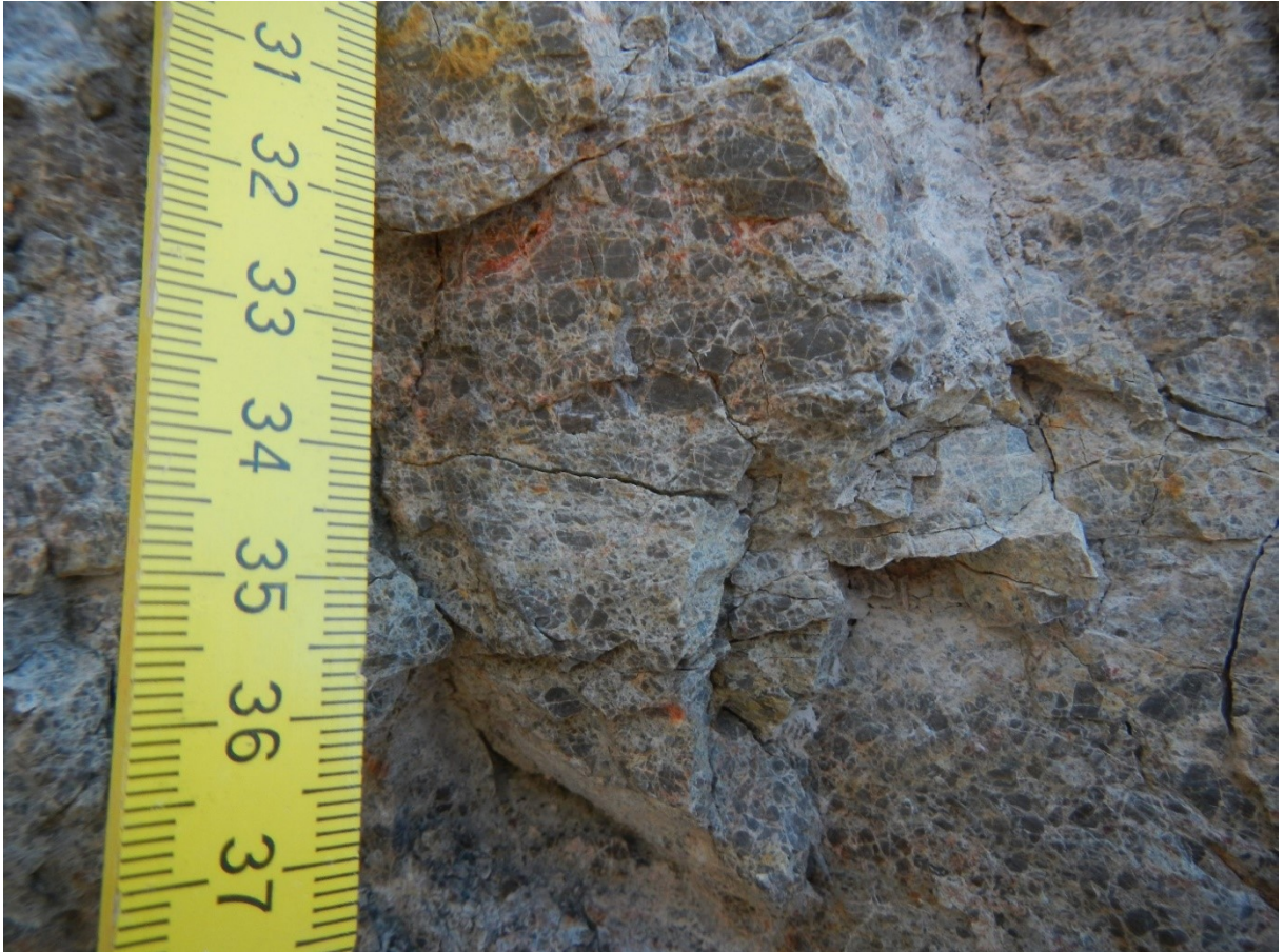
Figure 13: Dilation breccia with rock fragments showing jigsaw-puzzle-like fit of protolith components separated by matrix or cement were classified as dilatational breccia.
