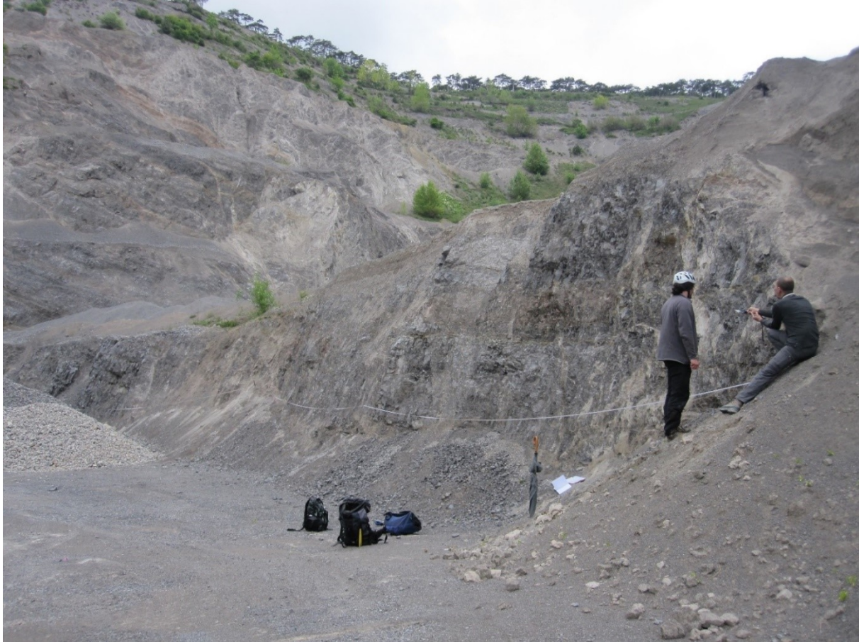
Figure 5: Strike of the first section of scanline 1, which is intersected 36 fault planes.
