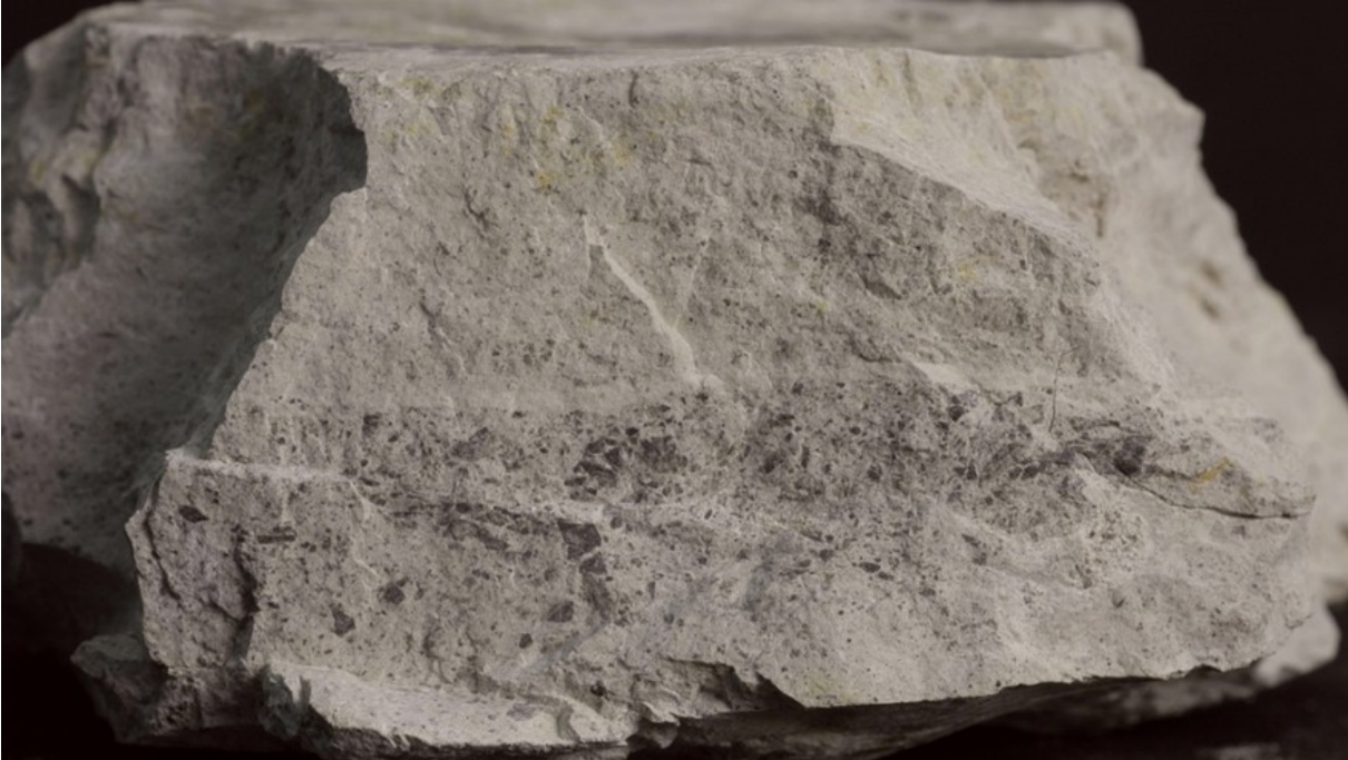
Figure 55: Sample 5.2. A plane of ultra-fine mature cataclasite, likely a former PSS, separates two zones of different matrix/protolith ratio and protolith grain size. Length of sample = 12 cm.
