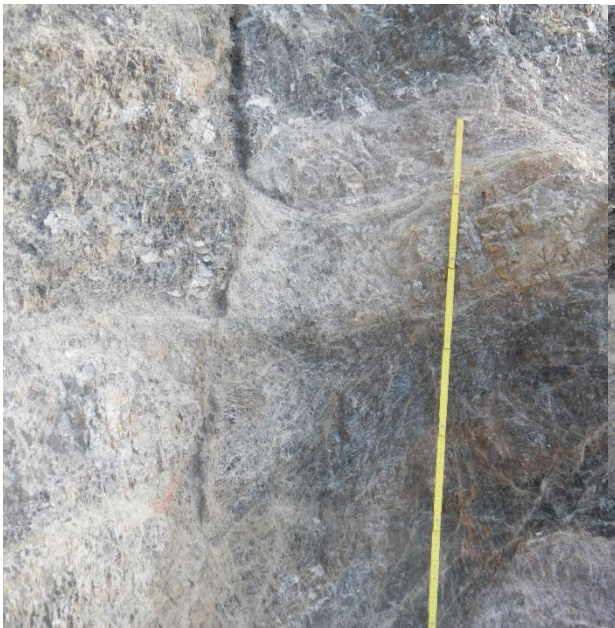
Figure 33: A category 5 normal-fault offsetting red marker beds divided by a category 1 flat
