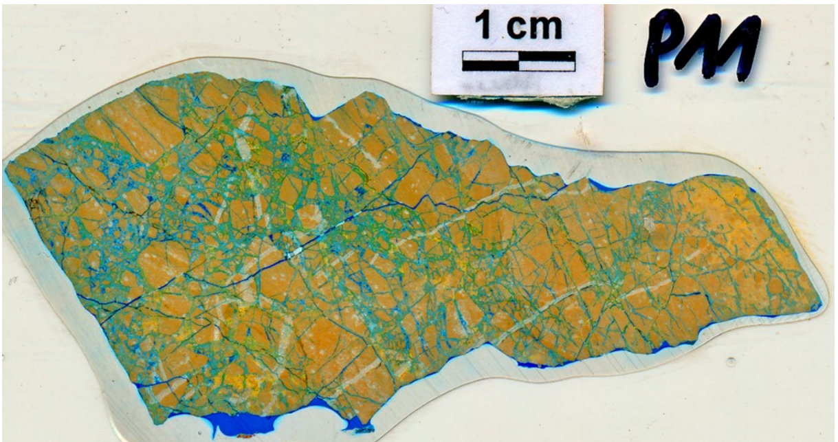
Figure 71: Section of sample 11. Note the fine network of younger fractures filled with porous material only rarely offsetting cemented older ones.
