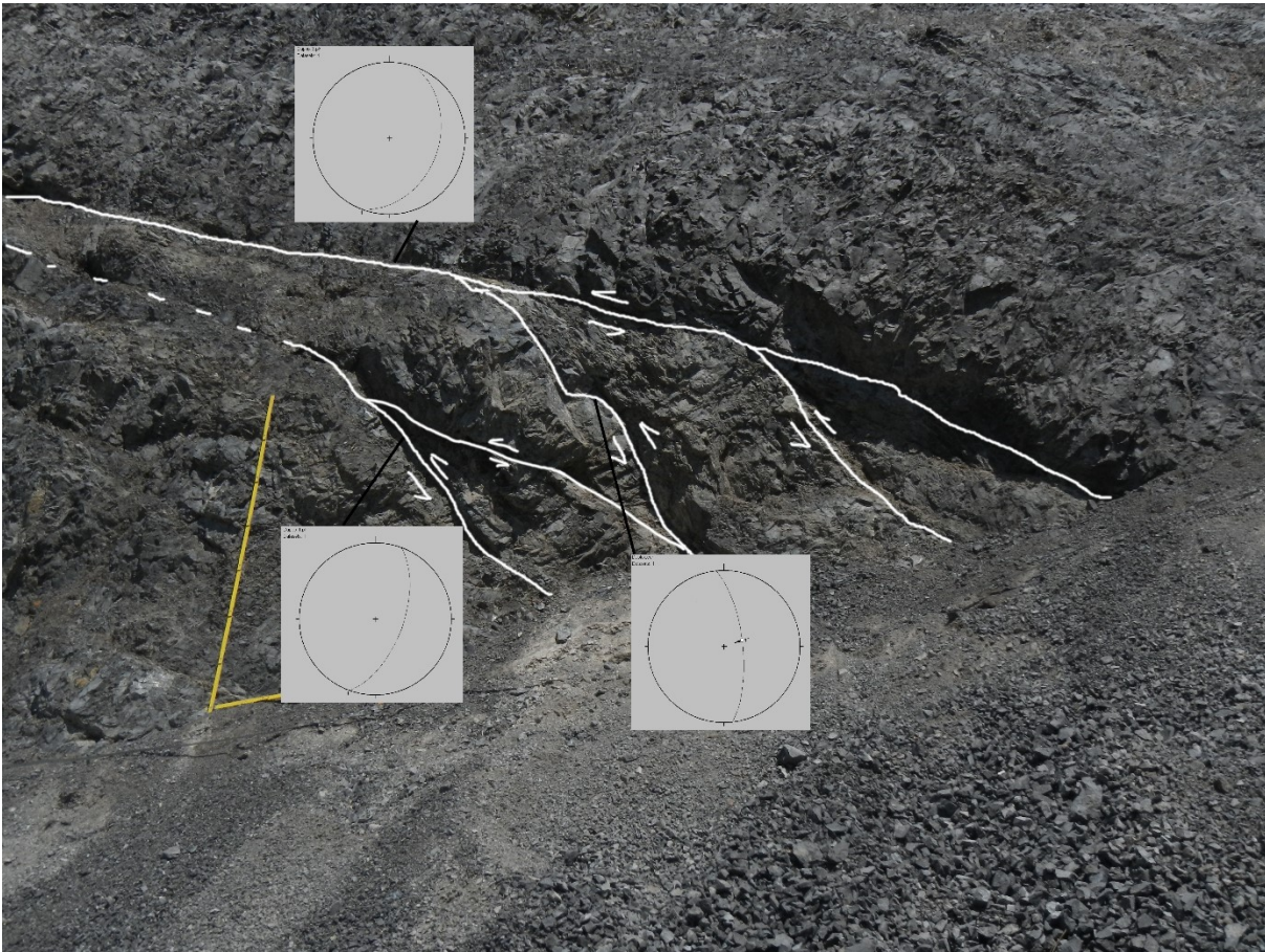
Figure 22: Structures interpreted as duplexes here with reverse faulting as the assumed process. Compare with the plot of all faults associated with this category and with the lineaments measured on faults all over the quarry.
