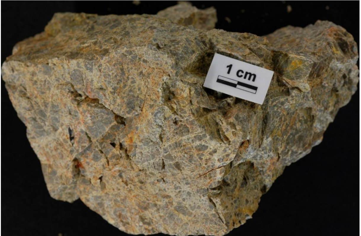
Figure 70: Sample 11 Jigsaw-puzzle-like fit of protolith grains in a "dilation breccia".
