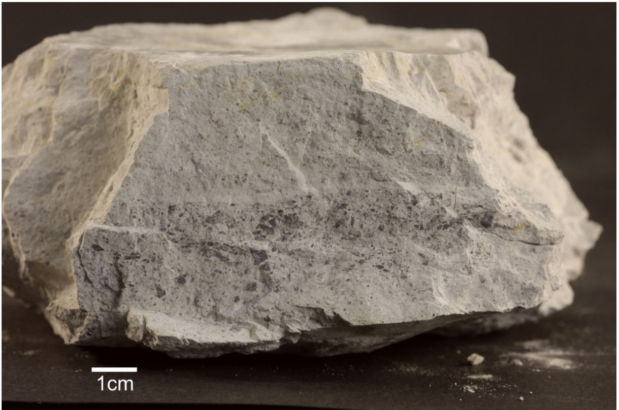
Figure 11: Matrix supported fault rocks were classified as cataclasites for the porosity estimation.
