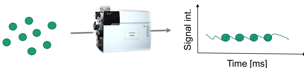
Figure 4: Schematic illustration of conventional ICP-MS. Dissolved ions yield a constant signal at the detector, usually resolved in millisecond dwell time.
