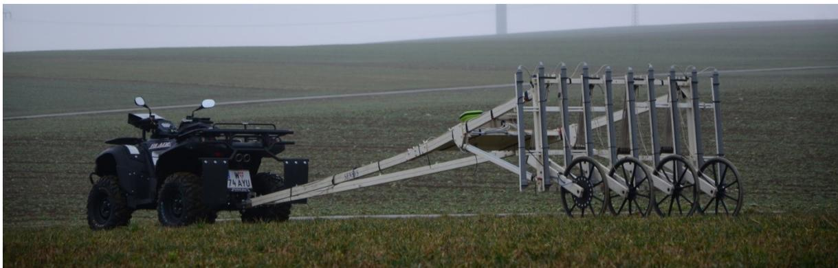
Figure 51: Motorized magnetic prospection. The multi-sensor array is towed by an ATV (© M.Kucera).
