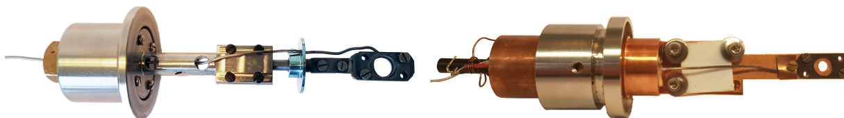
Figure 4.2: Left: Standard sample holder for measuring at room temperature and for heating the sample. Right: Cold finger for measuring in cooling mode.
