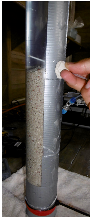
Figure 3. Image showing the sampling of pore water from sediment cores. The Plexiglas tube was sealed with waterproof tape before forcing it into the sediment. Pore water was taken with Rhizon MOM samplers (Rhizosphere) connected to a syringe. For oxygen measurements, a flow-through optical oxygen sensor (PreSense Precision Sensing) was connected in between.
