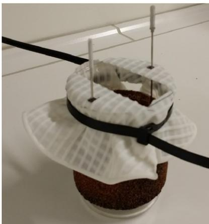
Figure 4. Electrodes fixed by a silicon mesh
