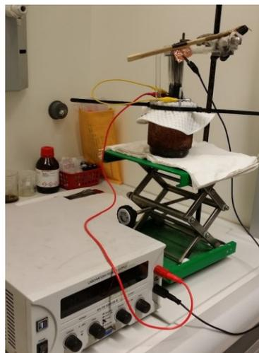
Figure 5. Setup for coating fibers
