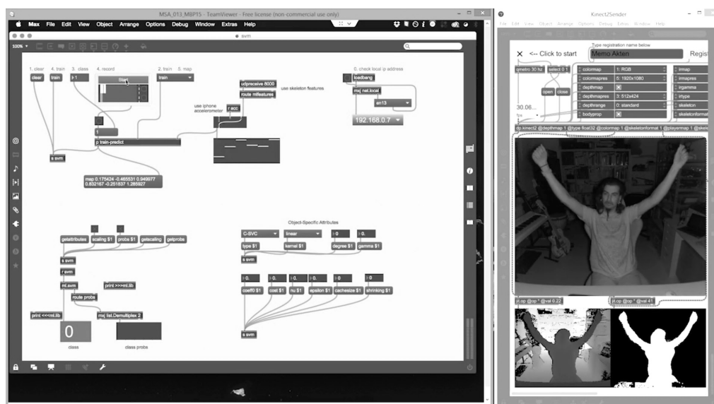
Figure 2.16. Max/MSP user interface, an example project recognizes gestures using Kinect device. Screenshot of the video Pose and Gesture Recognition using Kinect 2 skeleton tracking and Machine Learning Techniques in Max MSP Jitter - Vimeo , by M. Akten, 2015. Copyright by M. Akten.
