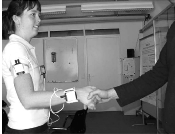
Figure 2.4. Accelerometers attached to participant’s lower and upper arm. Adapted from Gesture spotting with body-worn inertial sensors to detect user activities , by H. Junker et al., 2008. Copyright by Elsevier Ltd.
