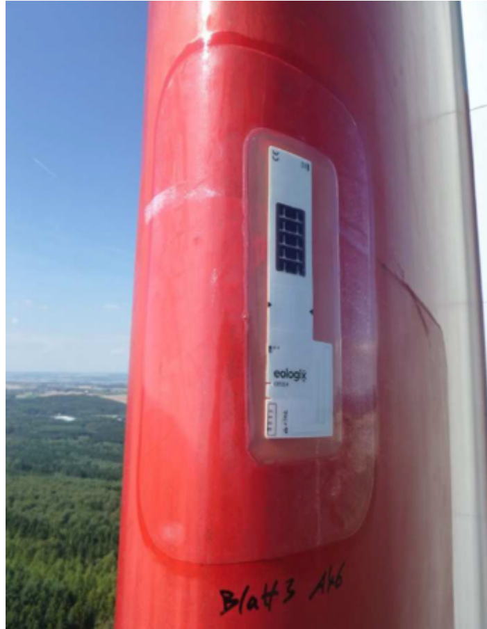
Figure 12: eologix sensor on the leading edge of the rotor blade (Burchhart, 2017).
