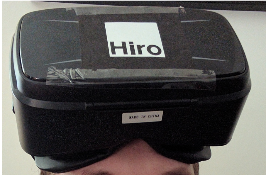
FIGURE 3.12: Photo of the test AR marker "Hiro" for VR headset tracking
