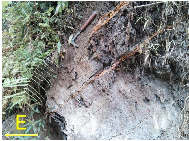
Figure 124: Two fractures penetrating the clay layers and filled with iron rich fluids
