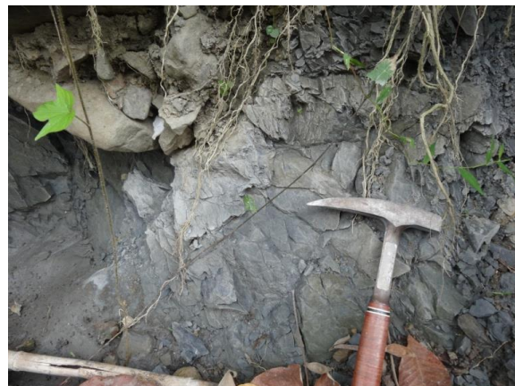
Figure 96: Very weak clay sediments in the underground
