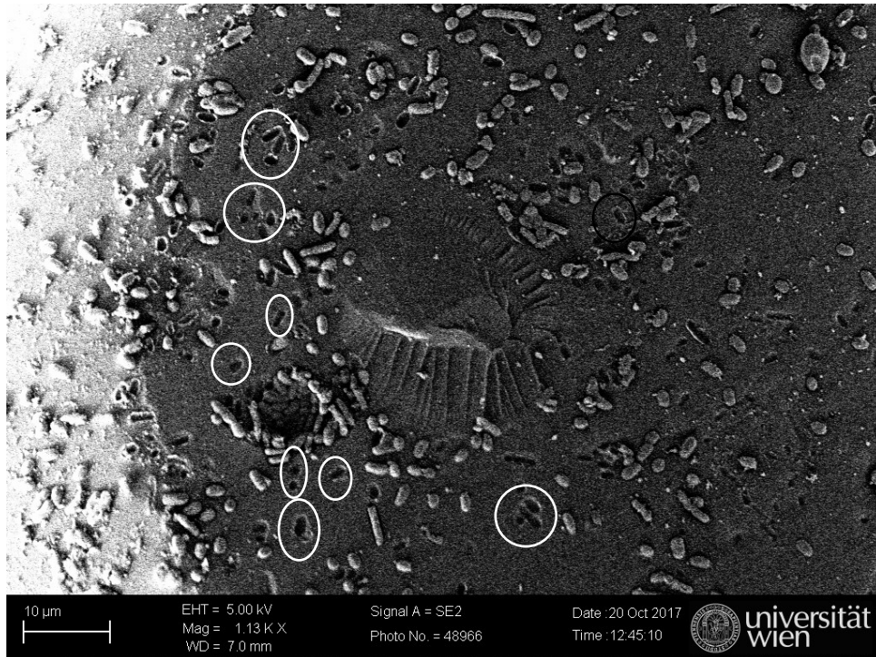
Figure 30: SE2 detector image of beads treated with a mixture of 100 mM NaCl and 1% SDS solution, some cavities are circled in white
