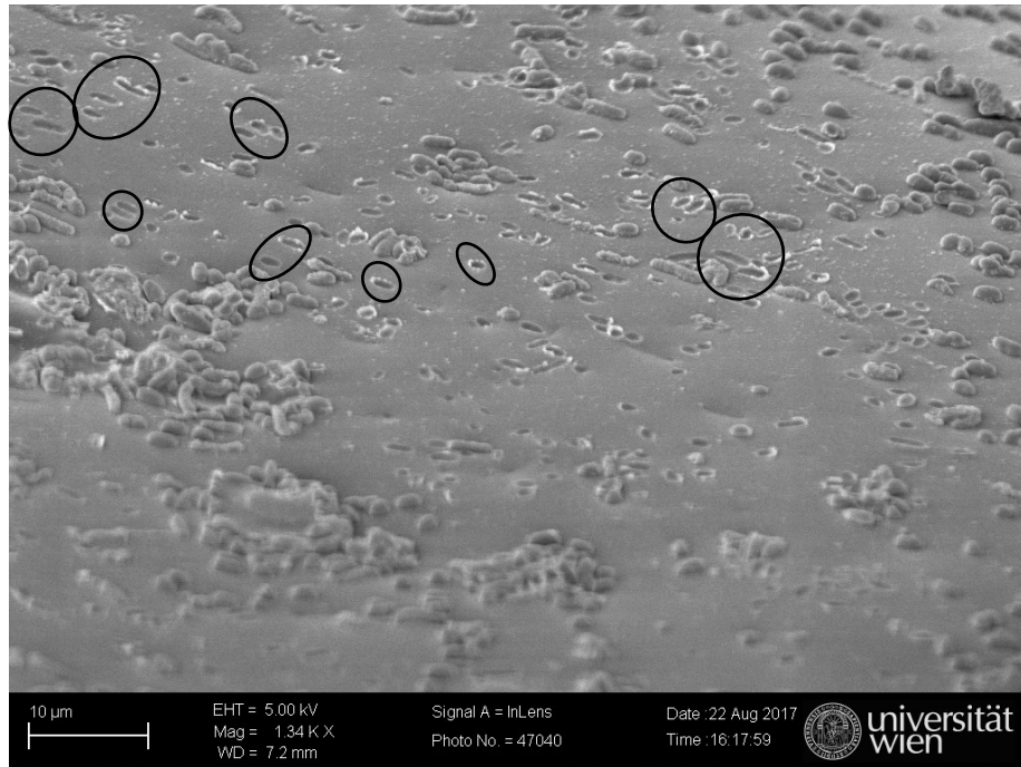
Figure 27: In-lens detector image from beads treated with a 3% glutaraldehyde solution, cavities of removed E. coli bacteria cells are circled in black
