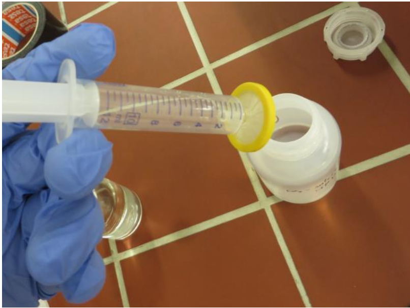
Figure 1: The picture shows the filtering of the suspension through the syringe filter (0.1 \mu m Millex) (Source:Sebastian Pontz)
