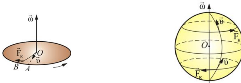
Figure 4: Rotating disc (left), Coriolis force acting on objects that move along the meridian (right). Source: http://ens.tpu.ru .
