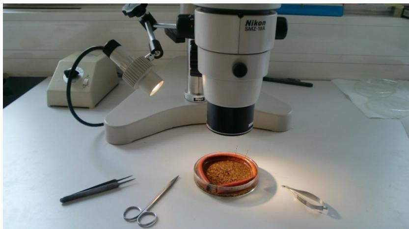
Figure 3 Preparation tools and reflected-light microscope
