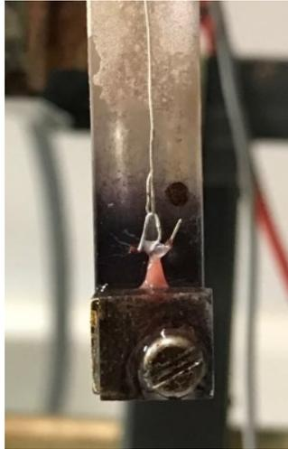
Figure 14 Musculus papillaris sandwiched between a platin electrode and a plexiglass
