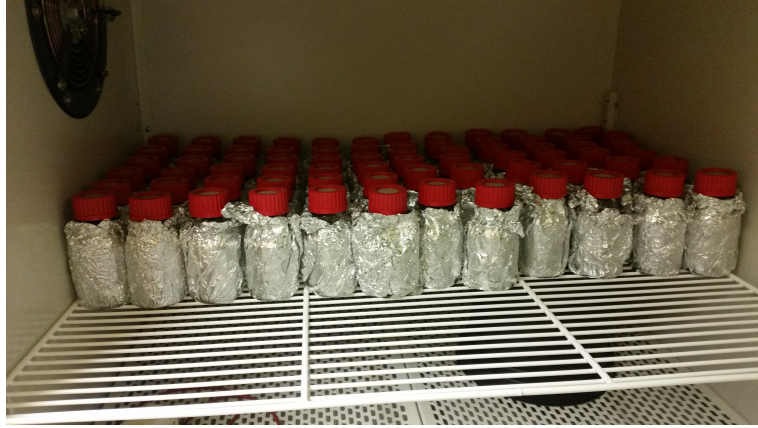
Figure 10: A photo of incubated peat samples. Jars containing peat samples with various water and fertilizer treatments in a chamber set to maintain 20° C. Jars in the photo are closed with lids, indicating that gas emission measurement is in process.
