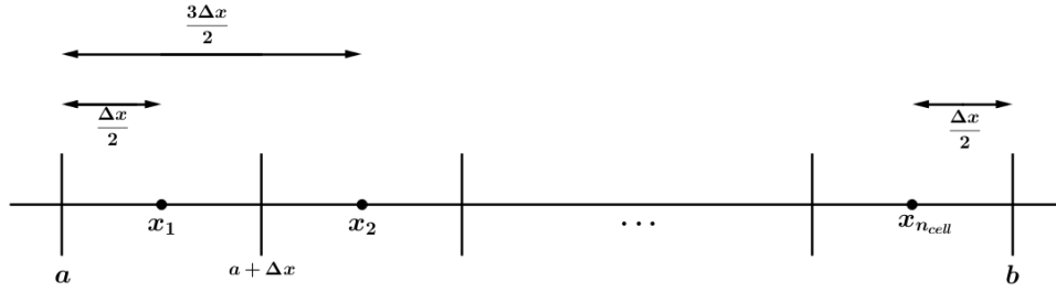
Figure 2.1: Illustration of the cell size \Delta x of a computational domain on the interval [a, b] .
