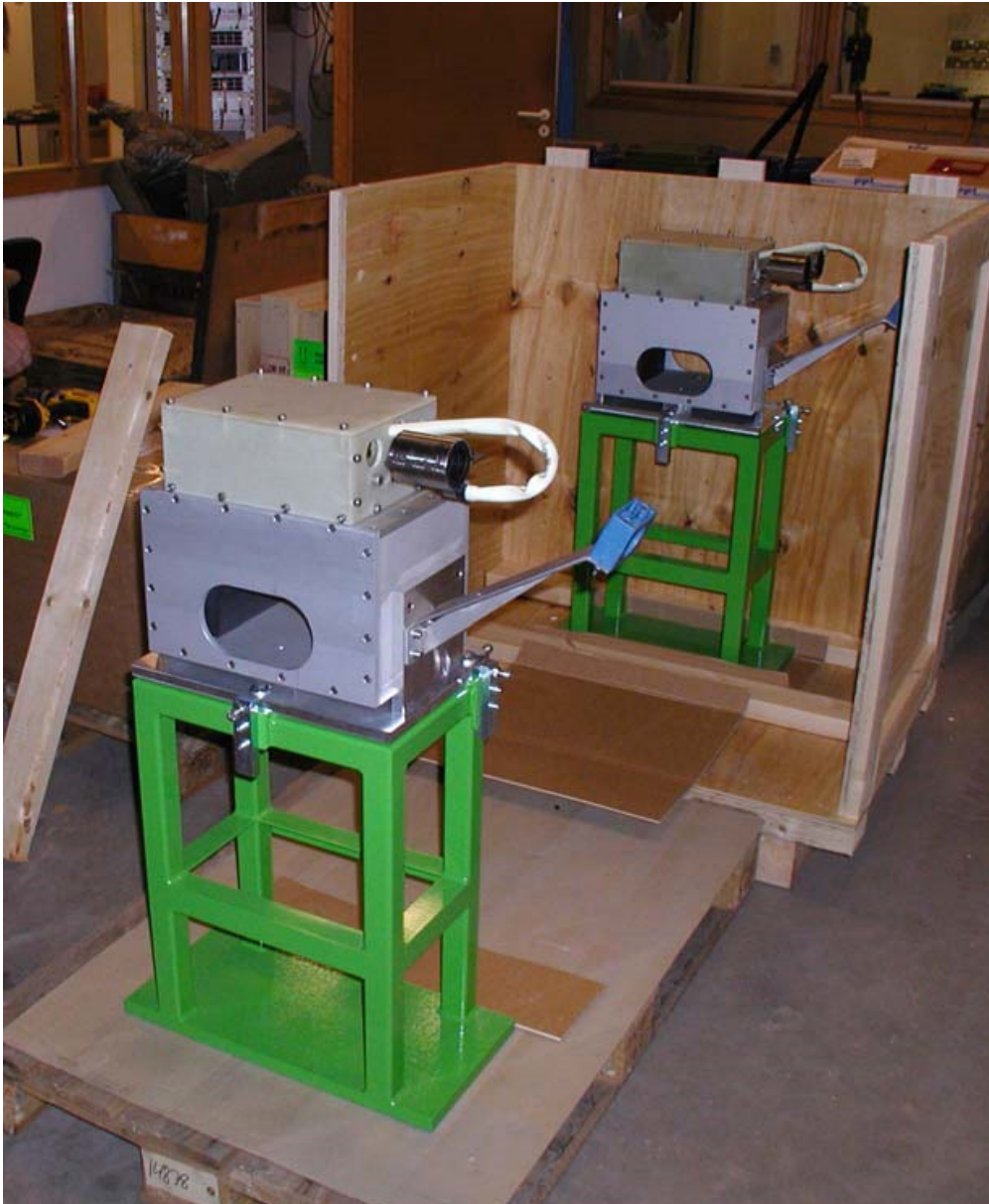
Figure 40 - Complete Assembly of the CNAO dump bumper magnet.
