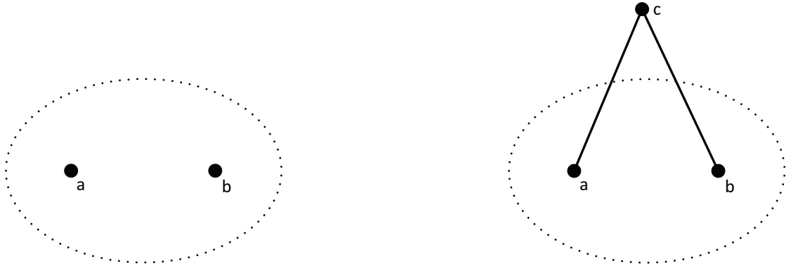
Figure 4: The first Henneberg rule: given any two vertices a and b (which may be connected by an edge or not), we add a vertex c and the two edges \{a, c\} and \{b, c\} .
