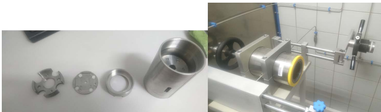
Figure 4 Clamp used to hold the DAC (left). Autoclave pressure chamber (right).
