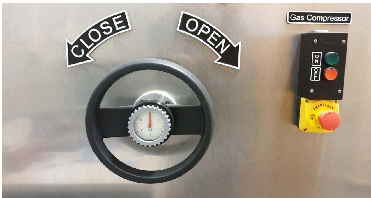
Figure 5 The wheel used to close DACs while inside the pressure chamber and the rotation indicator. ©Stefan Knesz
