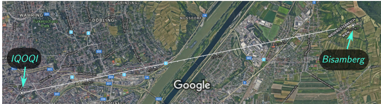
Figure 2.2: Satellite picture of Vienna from the free-space link of 10km between sender ( IQOQI ) and receiver ( Bisamberg ).
