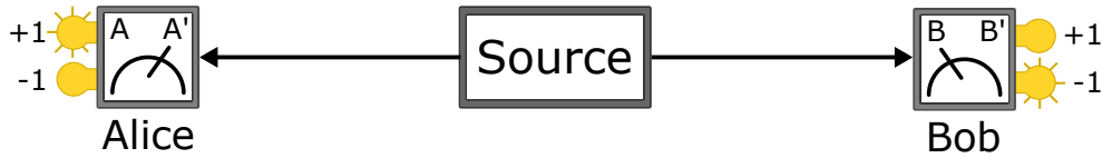
Fig. 2.2: Schematics for a Bell-type experiment. A source located in the center distributes particles to Alice on the left and Bob on the right. Both parties are equipped with a suitable detector which can be set to measure one of two properties \hat{A}, \hat{A}' and \hat{B}, \hat{B}' of the particle. Alice and Bob can freely choose their setting but are not allowed to communicate. Every time the detector measures, it gives out a binary output \pm 1 depicted by the two light bulbs at the side of the detector. After the experiment, Alice and Bob compare their results and compute the correlation parameter C . If the measured particles are at most classically correlated, |\langle C \rangle|_{\text{Cl}} = 2 . If the source emits maximally entangled particles, |\langle C \rangle|_{\text{QT}} = 2\sqrt{2} , violating the classical bound.
