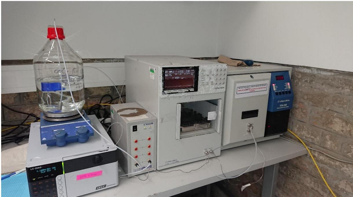
Figure 2.5: Photograph of the GPC setup.
