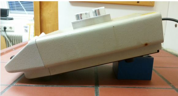
(c) The aluminium block (Fig. 4.1b) in a tilted heating plate, to ensure optimal matrix formation at 60-80 °C.
