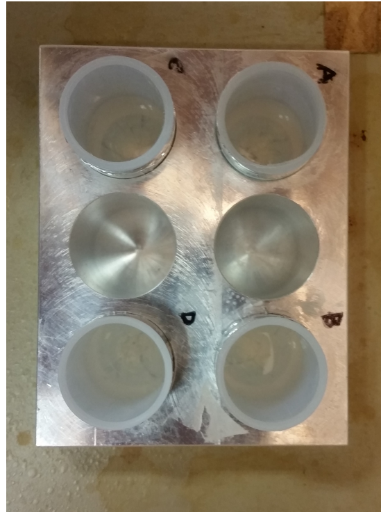
(b) Aluminium block with four vials for homogeneous temperature distribution. Vial positions marked A, B, C and D.
