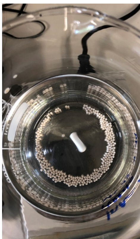
Figure 7: Curing of the pellets in distilled water on a magnetic stirrer.
