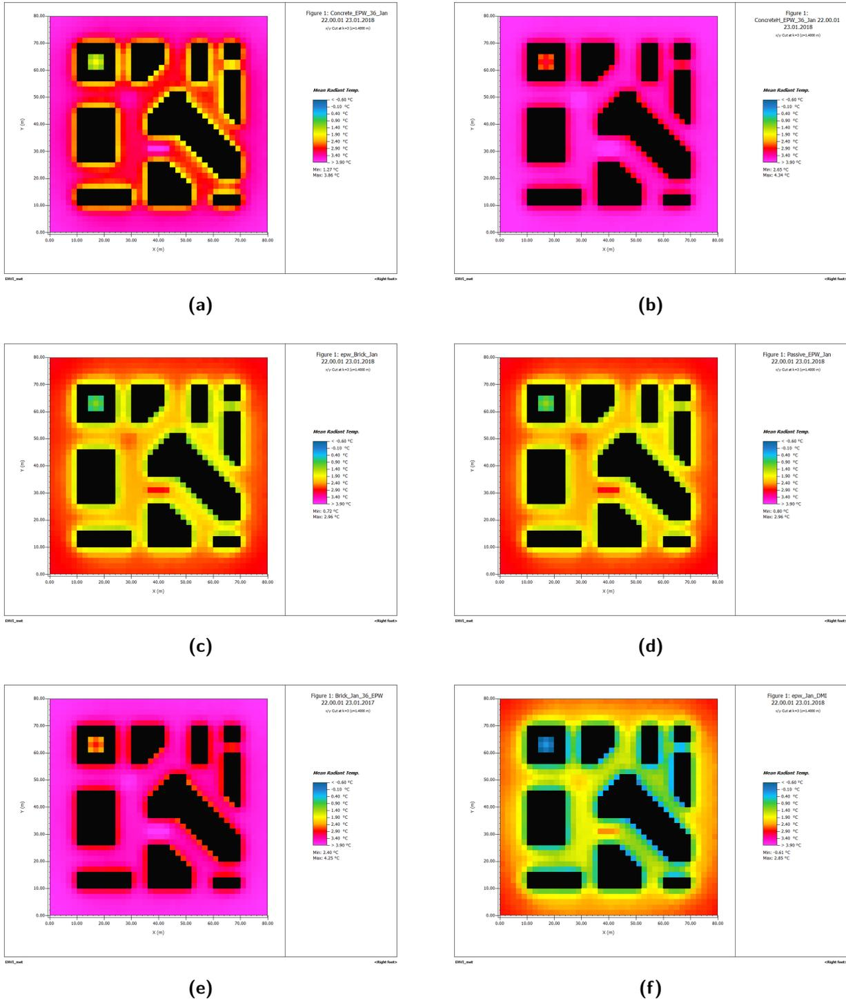
**Figure 7.10.** MRT (°C) of the different wall materials at 1.4 m height at 22:00 - concrete (a), hollow concrete (b), no-insulation (c), passive-wall (d), glass (e), moderate-insulation (f)
