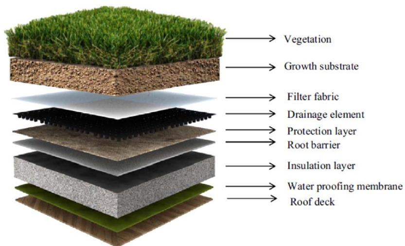
**Figure 4.4.** Construction of green roofs (Besir & Cuce, 2018, P. 917)
