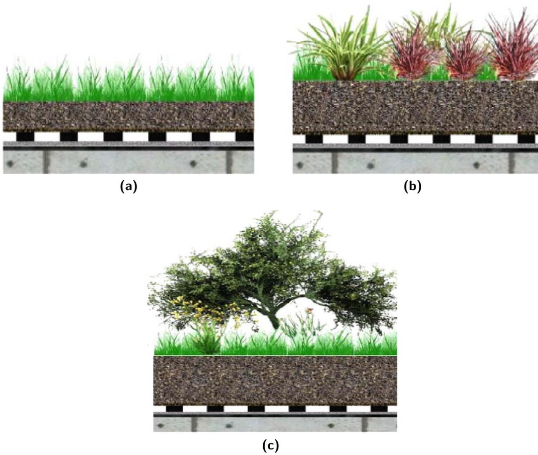
**Figure 4.3.** Different types of green roofs: Extensive (a) Semi intensive (b) Intensive (c) (Besir & Cuce, 2018, P. 918)
