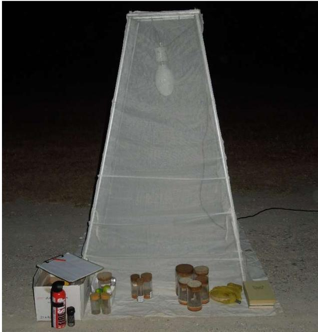
Figure 6.1: The light trap used in this study.
