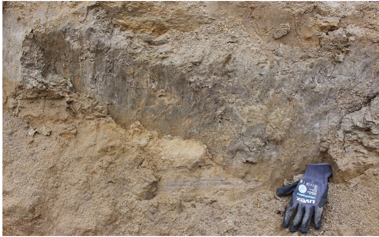
Figure 3.38.: Slickenside with lineation, S wall of building pit, glove (size 8) for scale.
