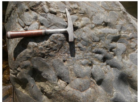
Figure 3.8.: 'Conglomerate' with dark blueish and grey-blueish clasts in grey brownish matrix
