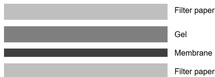
Figure 5: Structure of the "blotting sandwich"
