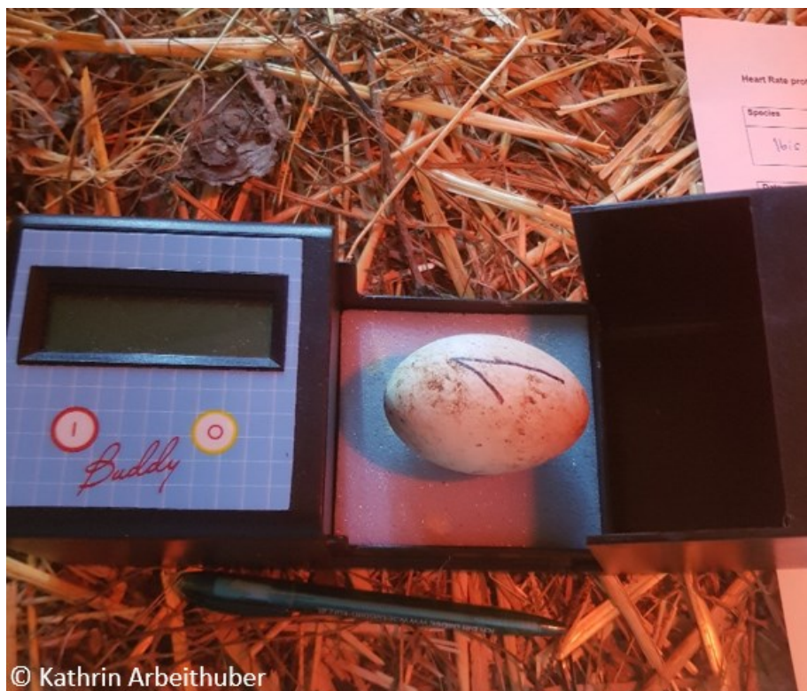
Figure 2: Heart rate measurement of an embryo with the digital egg monitor system “Buddy”
