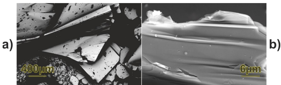
Figure 43: Misfit layer compound in the Se-Sn-V system; (a) large MLCs' crystals growing from the sintered powder pill of sample Sd58; (b) delamination of MLCs' due to mechanical stress yields thin and rippled layers.
