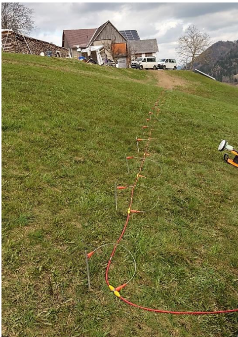
Figure 11: ERT cables along the Hofermühle, NÖ (March 2019)
