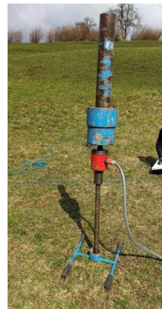
Figure 13: Dynamic penetration test (March 2019)
