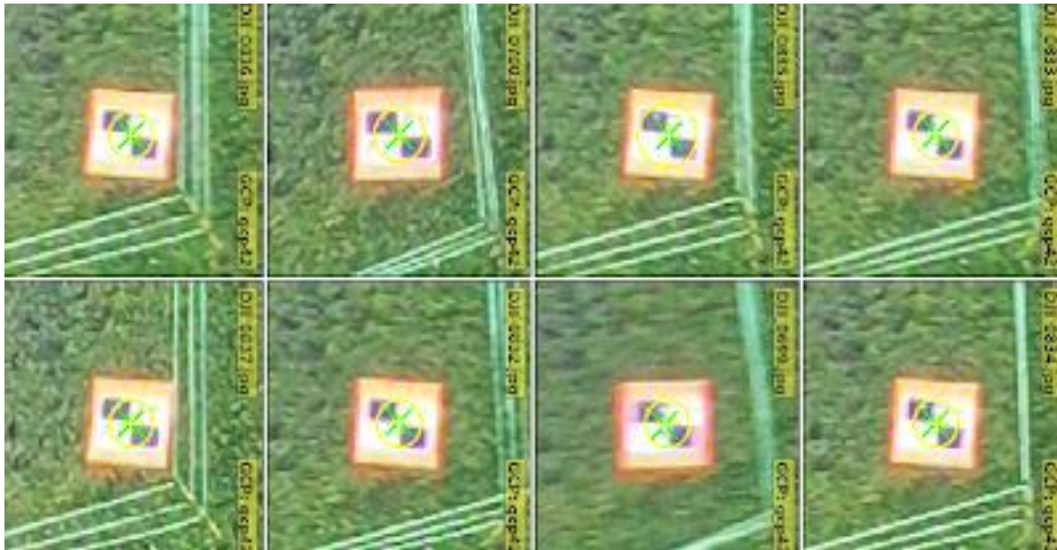
Figure 42: representative example of manual GCP marking on eight different images.
