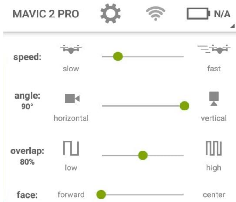
Figure 39: representative settings for a UAV-survey (taken from Pix4Dcapture 22.02.2021)
