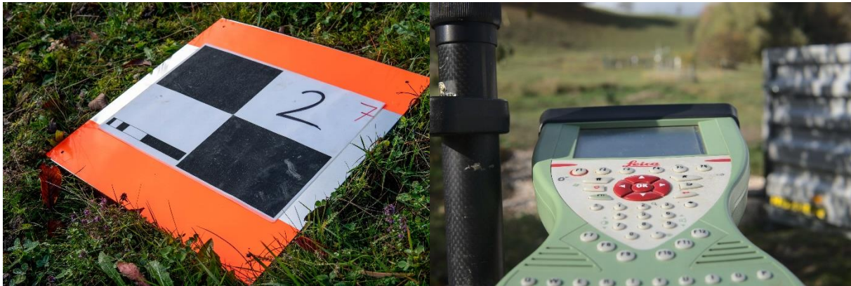
Figure 38: GCP with metal plate (left), Leica GNSS system (right) (05.11.2020)
