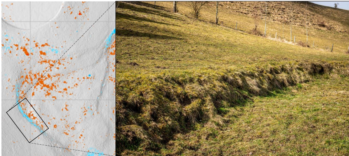
Figure 67: Close-up view of main scarp, southwest direction; DoD 18.11-23.04 (left) and photography taken on the 22.02.2021 (right)
