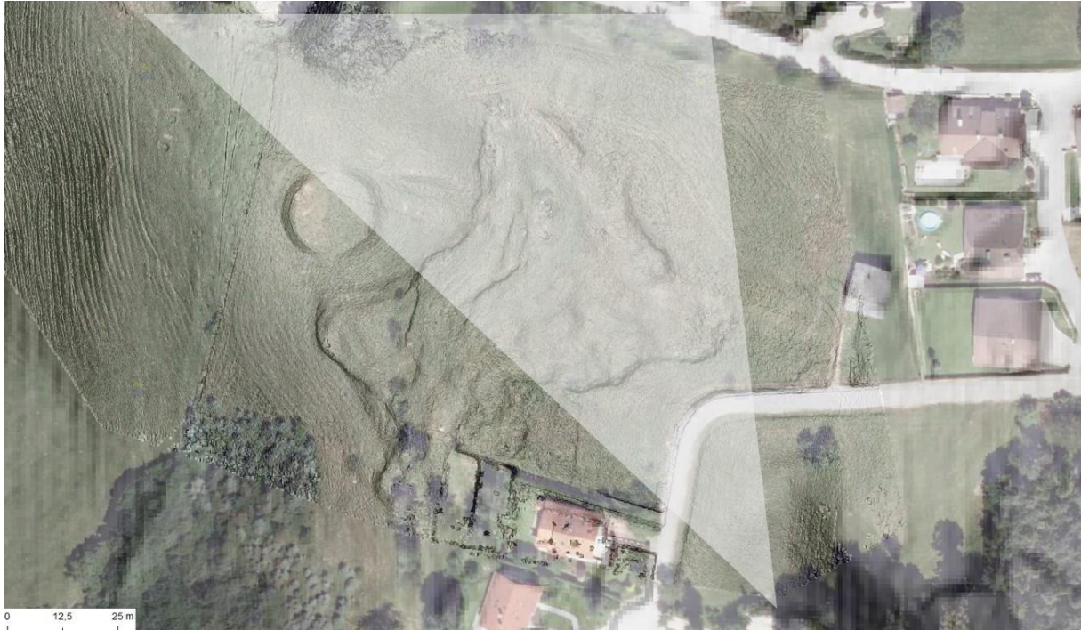
Figure 31: Area covered by the permanent TLS scanner at Salcher landslide POV (University Vienna 2021)
