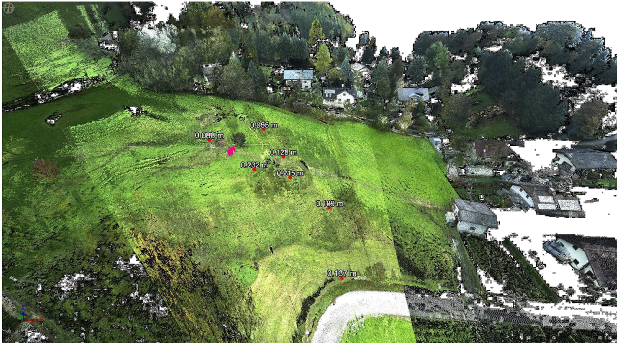
Figure 35: pTLS-data; distance measurements 2016-2019 (GLADE et al. 2019)
