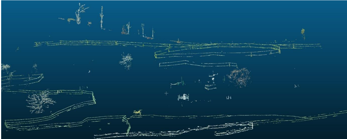
Figure 46: CSF off-ground points - removed for further analysis (representative example)
