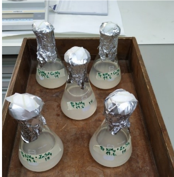
Fig.4 Prepared agar medium in flasks before sterilisation
