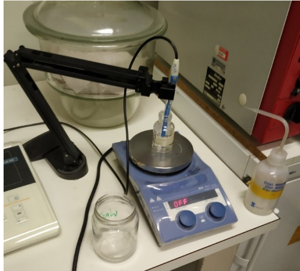
Fig.7 pH meter set up for calibrating pH of the fixative
