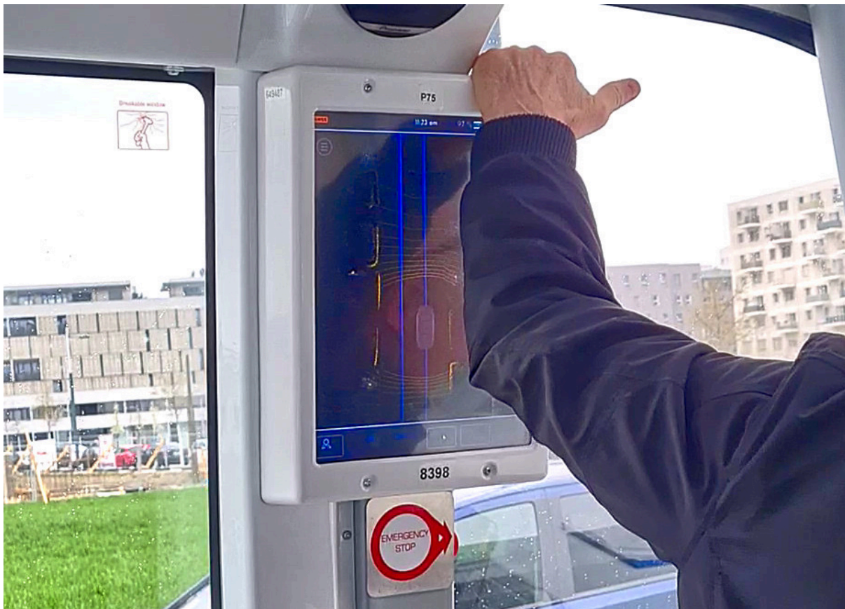
Figure XV: This interface shows the blue paths the bus followed, as well as the visual representation of the point cloud matching technique.
