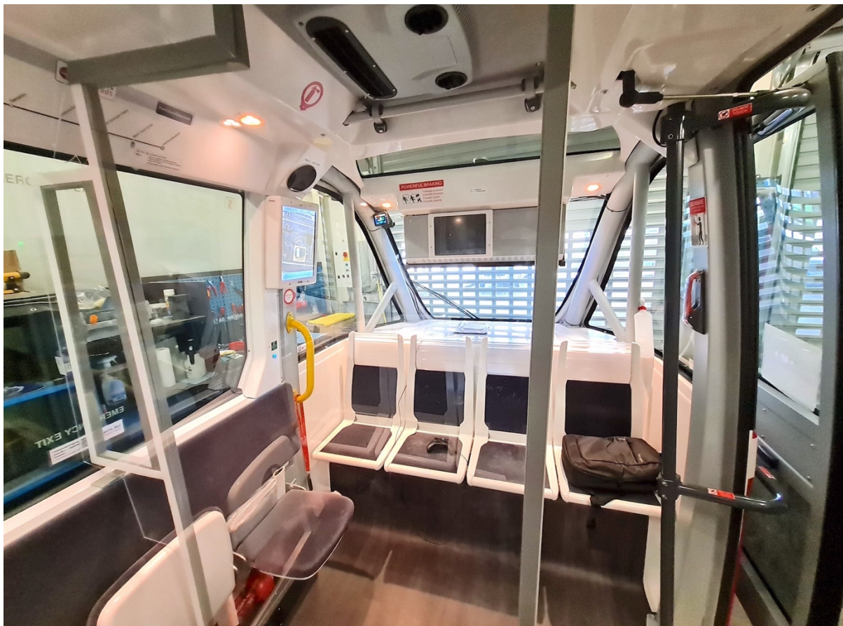
Figure XIII: The interior of the bus. Note the XBOX gamepad lying on the seats, which was used for manual driving, and the terminal screen.
