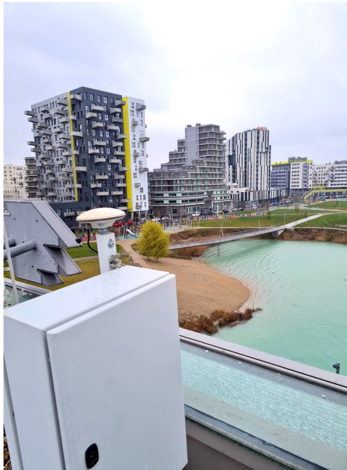
Figure XVI: View from the roof of the metro station. The device in the foreground is the GPS reference antenna.
