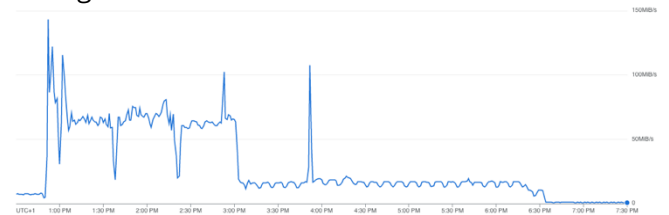
Figure 8 Figure 9. Read data rate during ingest (MiBytes/sec)
