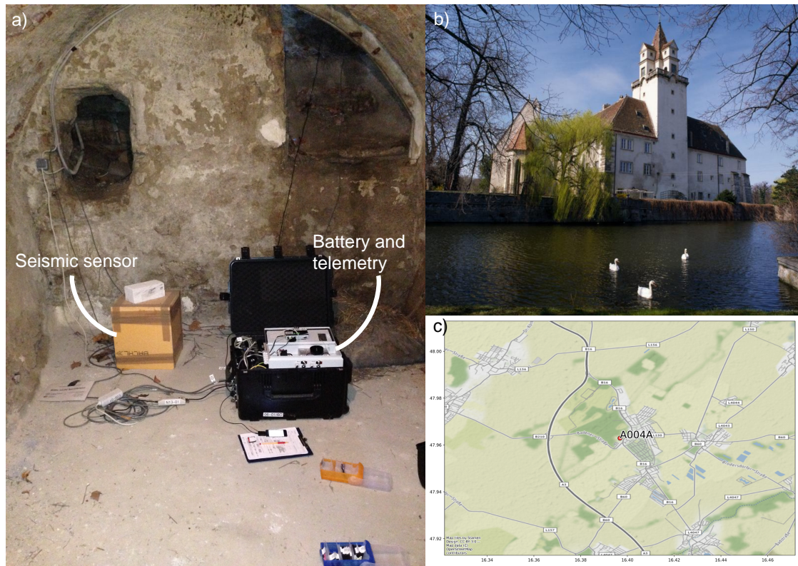
Figure B.2.: Typical seismic station of AlpArray (A004A). a) Setup of a seismic station. Seismic sensor is confined within the brown box and connected to the black box with batteries and telemetry. b) Building, where the station is located (in the basement). c) Map displaying the position of the seismic station.
