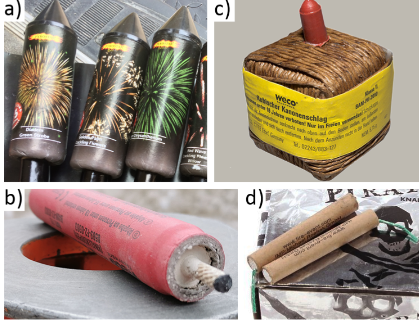
Figure 2.4.: Explosives used for the experiment. Left: a) "Small" charge (0.80 g NEM), b) "Medium" charge (6.75 g NEM), c) "Large" charge (7.50 g NEM), and d) Rocket charge (75 g NEM).
