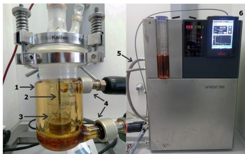
Fig. 27: HT-TIPS setup. On the left figure: glass vessel (1), thermometer (2), 50 mL glass beaker with polymer/solvent solution (3), high temperature hose connectors (4). On the right: pipes connected to tap water (5), Huber Unistat T305W HT thermostat with PILOT ONE control unit (6).
