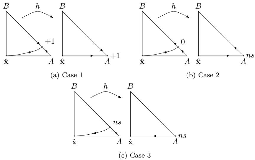
Figure 11: In Case 1, the equilibrium  $\mathbf{p}_0$  is saturated before and after applying the homotopy  $h$ . The boundary index remains constant and equals  $+1$  since the equilibrium is locally asymptotically stable.
