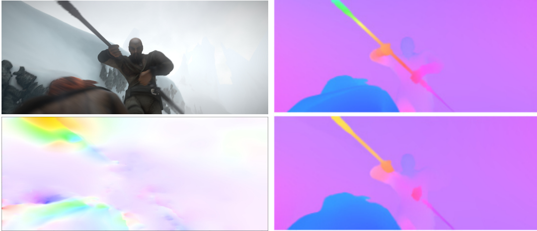
Figure 32: Ambush_3 Sequence [39]: frame 1 ( left-top ), ground-truth ( right-top ), computed flow algorithm (2) ( left-bottom ), computed flow RAFT ( right-bottom )
