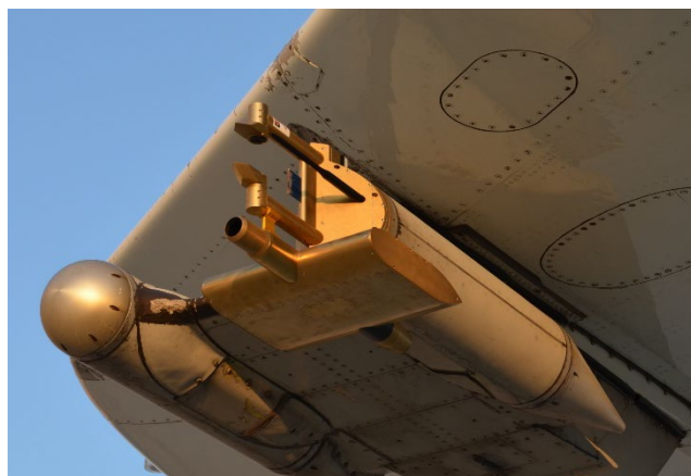
Figure I 2-1. The second-generation Cloud, Aerosol, and Precipitation Spectrometer (CAPS) instrument of University of Vienna mounted under the wing of the NASA DC-8 aircraft.
