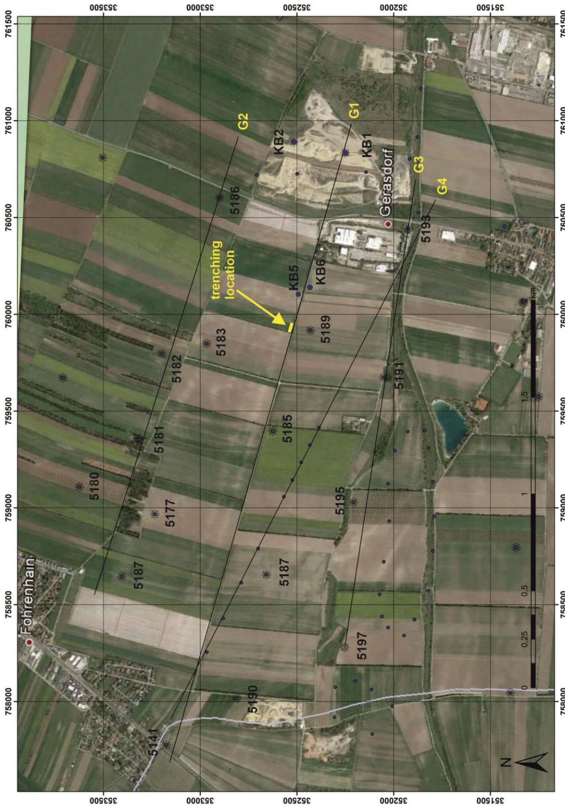
Fig. 4: Location of cross-sections G1 to G4 (black lines); trenching location in yellow; blue circles indicating blast holes; black crossed circles indicating boreholes from the ÖMV drillings collected in the HADES database and violet crossed circles indicating boreholes from KOVANDA GmbH.
