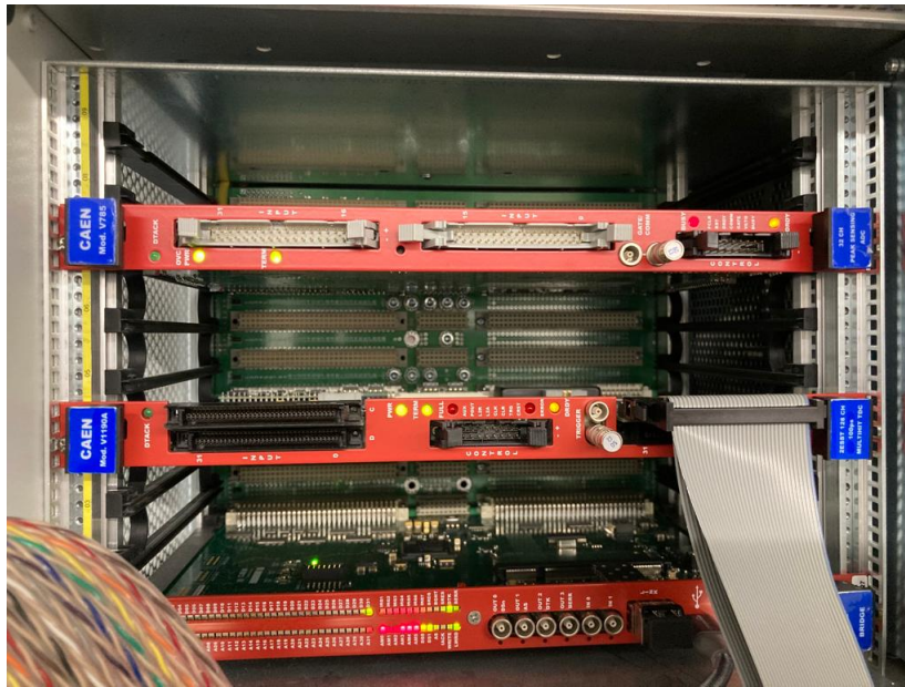
Figure 16: rack with inserted PADC (top module) and inserted TDC (middle module).
