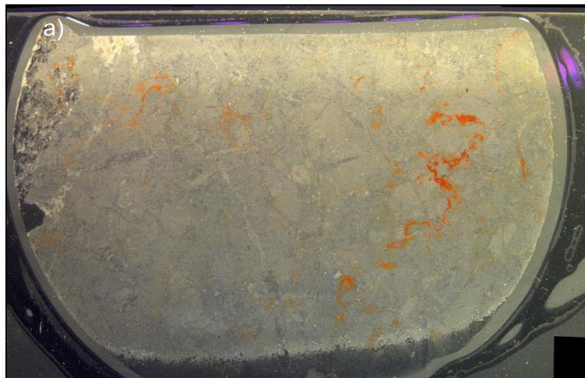
Figure 83: Cut-out from sample LP38 with Fluorol in pores and cleavages. As there were almost no spaces filled with Fluorol, the pore and cleavage space must be minimal. A stitching of the UV-light picture was not possible due to the low porosity. The sample is 1.5 inch wide.
