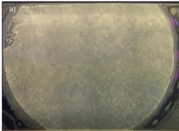
Figure 115: Cut-out from sample PW6/2 with Fluorol in pores and fractures. a) shows the sample under reflected light. There is no picture of the sample under UV-light because no stitch could be made from the almost non-existing UV-emission of this sample.
