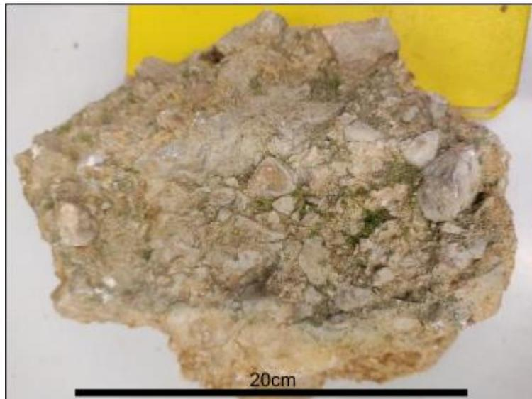
Figure 95: Handpiece of MT31, extracted out of a 1.5 m thick band of cataclasite, size: 1249 cc.
