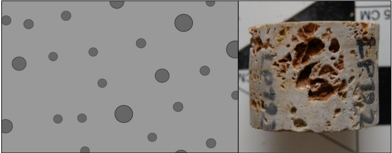
Figure 11: Left: Simplified two-dimensional view of rock sample with round (dark grey) pores on the surface. Due to the inability to hold water after extraction of the sample out of the water column, larger pores volumes directly on the surface do not get measured. Right: Example of LP19/2.5 with a possible high influence of this effect on the measured porosity.
