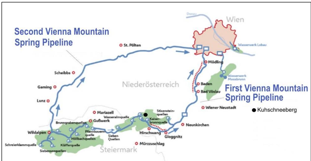
Figure 1: Map showing the two Vienna water mains connecting the city to springs and their catchment areas. The Kuhschneeberg (black dot) is located at a protective area (green zone) forming the catchment of some major tapped springs (like the Kaiserbrunn spring). Modified from Wiener Wasser, 2021.
