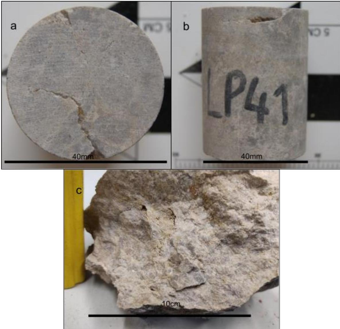
Figure 84: **a) and b)** 52,39 mm long core plug of LP41 in top view (a) and lateral view (b), the plug largely reminds of LP43 and LP36, **c)** Handpiece of LP41, there seem to be no fractures induced through the fault, size: 725 cc.
