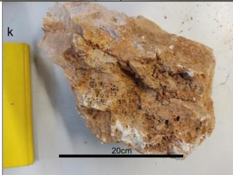
Figure 76: **i)** and **j)** 30,03 mm long core plug of LP19.2 in top view (i) and lateral view (j) with visible porosity. **k)** Handpiece of LP19.2 Wetterstein Formation (Karstified), the pores are often confined grid-like, the veins are more resistant to karstification and often build up the walls of the pores. size: 3154 cc.
