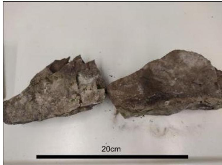
Figure 91: Handpiece of MT10 and MT10.2 Opponitzer Formation (Limestone), both samples have a sulphurous odour, size: 626 cc (MT10, left), 927 cc (MT10.2, right).
