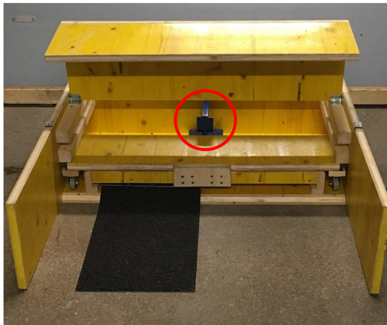
Figure 5: Configuration of the apparatus in the unsolvable condition from the pig's perspective. The red circle indicates the blue block behind the panel.
