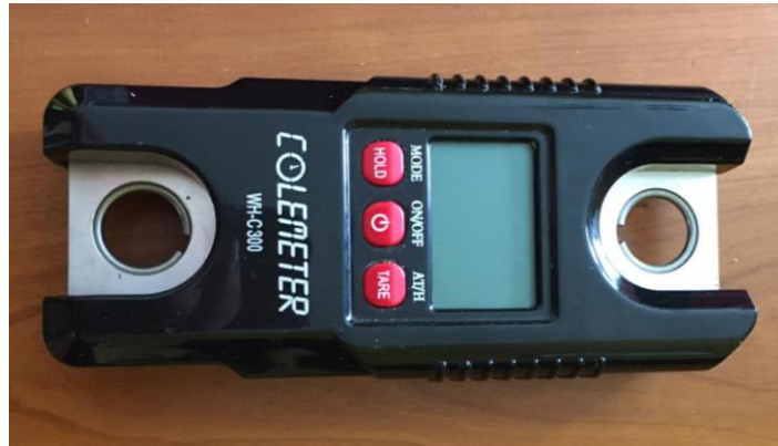
Figure 6: Picture of the scale used to determine the pigs' strength of pushing in the attached condition and to later keep the force of the experimenter's pulling in the foot discomfort condition at this value. Hooks and carabiners could be attached to the two ends of the scale to connect it to the chain.
