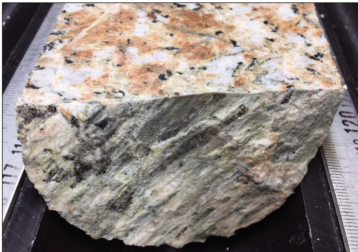
Figure 4.1. Perspective macrophotograph of a split core (granite lithology) from the IODP-ICDP Expedition 364. Core sections similar to this one were further cut at selected intervals, and the obtained samples were sent to the NHMV for investigations. The core width is 86 mm. From Morgan et al. (2017).
